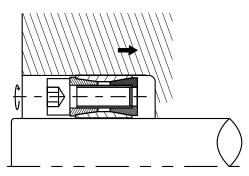
Put bolts into the corresponding threaded jack holes, turning the bolts clockwise, loosen the inner taper rings.
