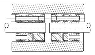
Mounted with shaft sleeves to connect transmission between two shafts.
