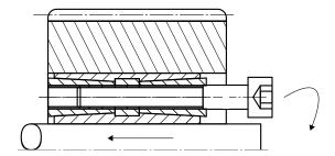
After removing the tight taper ring in A side, place the unloading tap hole in the middle ring, tightening and pres in proper order, separate the tightening taper ting in B side with the inside and outside taper bushes step by step from the other side.
