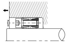
Pull out the bolts with strength, loosen and remove outer taper rings.
