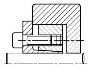
Installed with non-through bored hub, and positioned with hub end. The outer ring moves in axial direction during usage, thus inner ring and bore of hub will be tightened.
