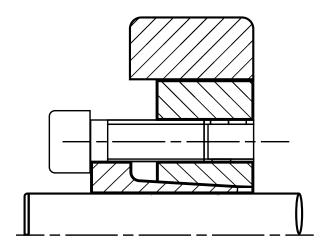
Positioned with hub end and then fix the position in axial direction. The outer ring moves in axial direction during usage, thus inner ring and hub bore will be tightened.
