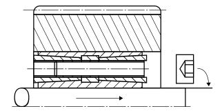
Loosen and remove all the tightening bolts first, then place the unloading tap hole of the tightening taper ring in A side, tightening and pressing in proper order, separate the tightening taper ring in A side with the inside and outside taper bushes step by step.
