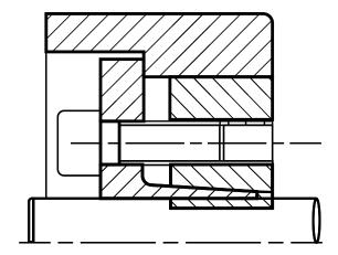
Installed with through bored hubs, in the form of step bored. It can be positioned in axial direction. The outer ring moves in axial during usage, thus inner ring and hub bore will be tightened.
